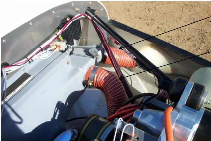
Figure 22. SCAT Hose Detail #1
